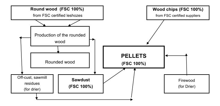
"Basic Timber Company" for the production of pellets uses:
